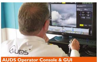
All the system elements of AUDS: Radar, EO System and RF Inhibitor are fully integrated into the operator console. The AUDS Operator Console requires a single operator and comprises two screens.
